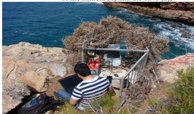
Figure 4. Mounted camera system directed to the cave
